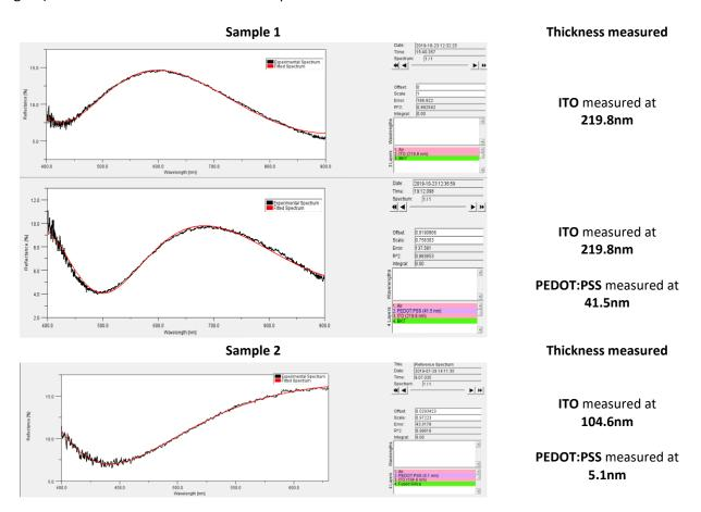
**Conclusions**: FR-pRo VIS/NIR tool was successfully used for the thickness calculation of conductive polymer films on transparent substrates with ITO.
